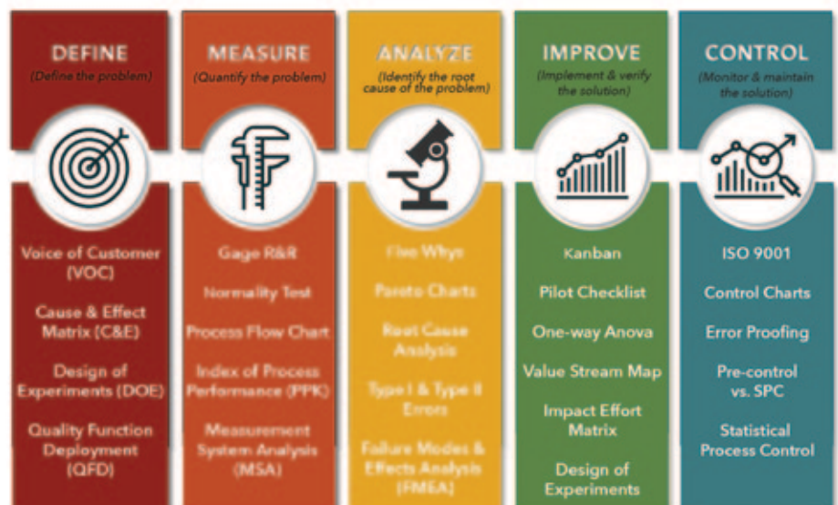
There are many tools that exist within each segment of the DMAIC method. Here are several applied to Six Sigma projects by Allied's candidates as they pursued their certification
